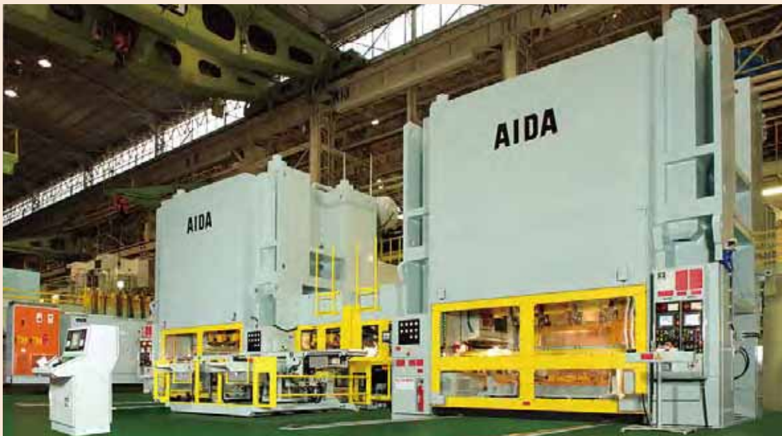
■ UL Series Tandem Transfer Line—High-speed synchronization of two 20000kN transfer presses
