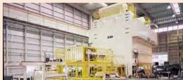
■ Transfer system with a new type of feeder for aluminum material
