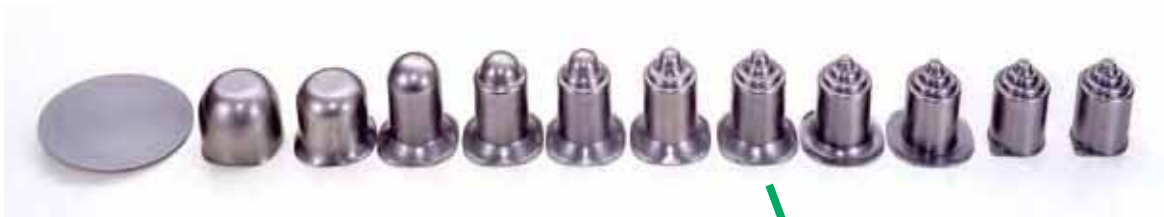
Automotive motor casing (total of 12 forming stages)
