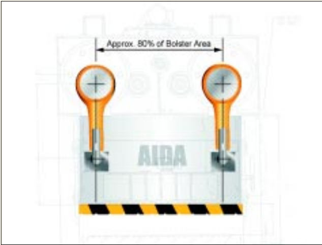
Caption: Wide spaced connections, approximately 30 percent farther apart than conventional presses, provides greater resistance to slide tipping caused by off center loads.
