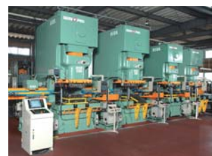
A tandem press line composed of four small general-purpose NC1-D servo presses and press-to-press A-8 transfer robots. It does not require major infrastructure equipment to install the equipment, and its small size also enables installation in factories with limited headspace. This is a solution that enables high-performance press metalforming even in a constrained environment.
