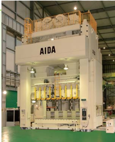
A 2,300-ton large servo press
