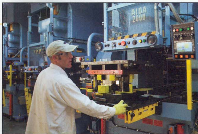
Figure 3. With the gap-transfer line, instead of one progressive die with five stations, Newman is able to use five single dies.
