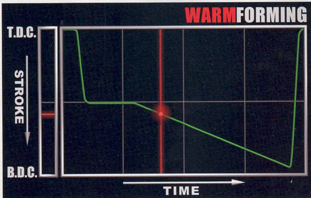
Figure 2—A graphical representation of the warm forming process on a servo-controlled press. The horizontal portion early in the stroke represents press dwell time. (T.D.C., Top Dead Center; B.D.C., Bottom Dead Center)
