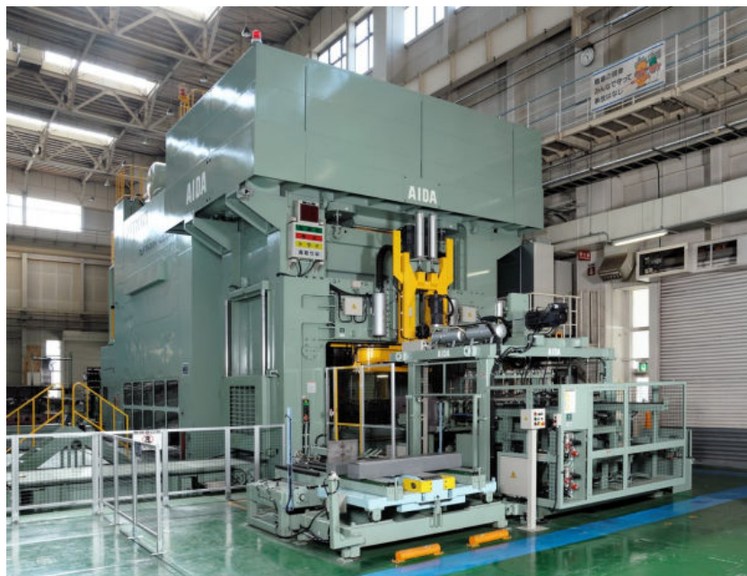
Foreground: SMX-10000(LD) dedicated high-strength steel forming press (Capacity: 10,000 kN) Background: Existing transfer press (Capacity: 15,000 kN)
