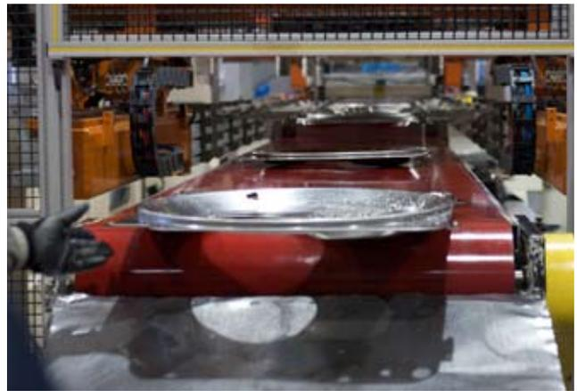
The Flextronics NST can accommodate up to seven dies on a bolster and transfer the part up to seven times. A variable position exit conveyor on the final transfer station is integrated with safety interlocks on the press control to allow the conveyor position to be linked to specific part numbers with specific numbers of stations.
