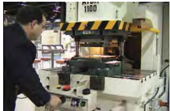
ServoPro’s hand crank feature allows manual progression through the slide motion ensuring die setup and synchronization of ancillary equipment is correct before production.
