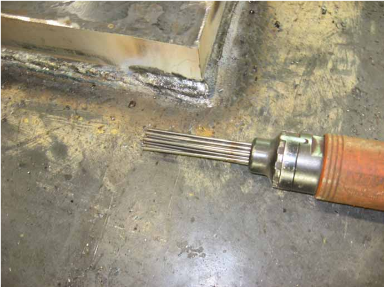
Air Needle Scaler for cleaning welds
