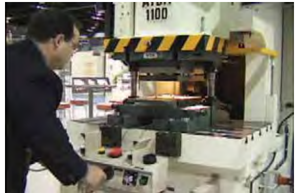
ServoPro’s hand crank feature allows manual progression through the slide motion ensuring die setup and synchronization of ancillary equipment is correct before production.
