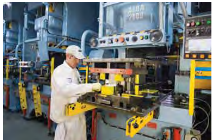
With the ServoPro gap press transfer line, instead of one progressive die with five stations, Newman is able to use five single dies.
