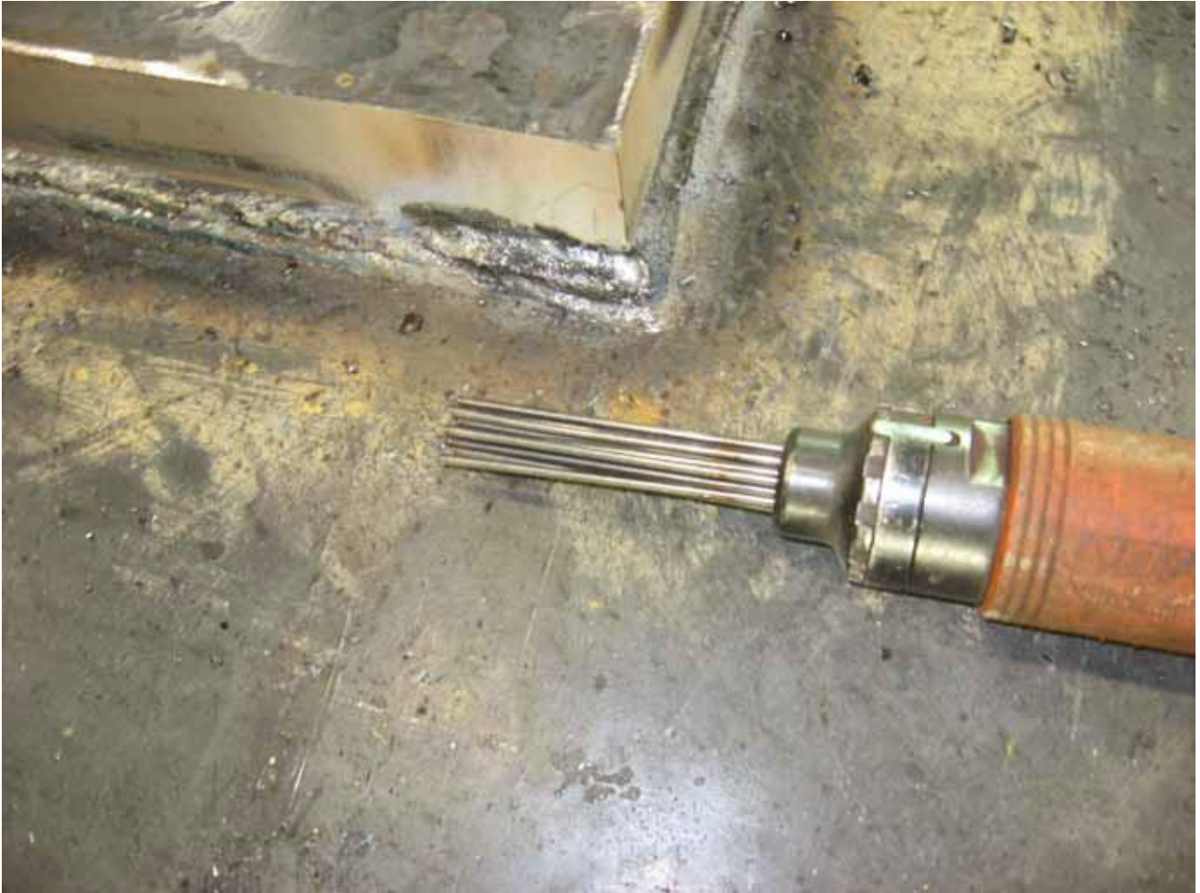
Air Needle Scaler for cleaning welds
