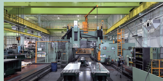
A large 5-face machining center for slides and beds, etc.
