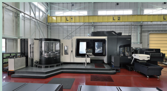
A state-of-the-art 5-axis machining center for high-precision components (DMC160FD/dB)
