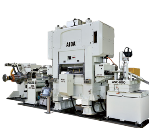
A High-Speed Precision Press Line for EV Drive Motor Cores
