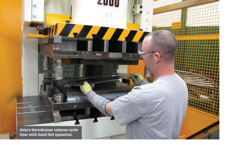
low speeds, the Aida DSF Series Servoformer allows the operator to run the press at a velocity as low as 1 spm during forming then return to full speed for the nonworking portion of the ram cycle without causing a drop in productivity levels.
