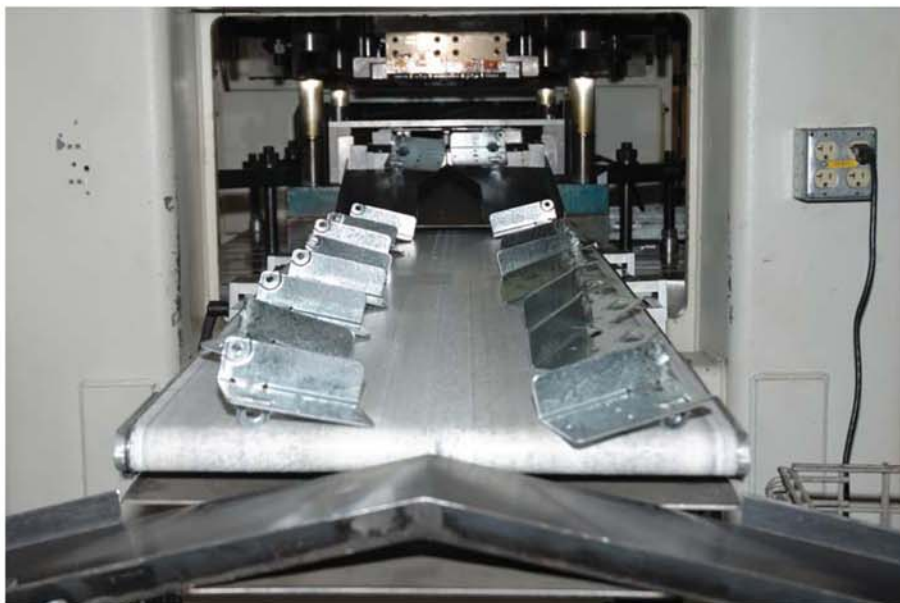
The NSU's low deflection and overall accuracy allows C.H.I. to manufacture burr free parts.
