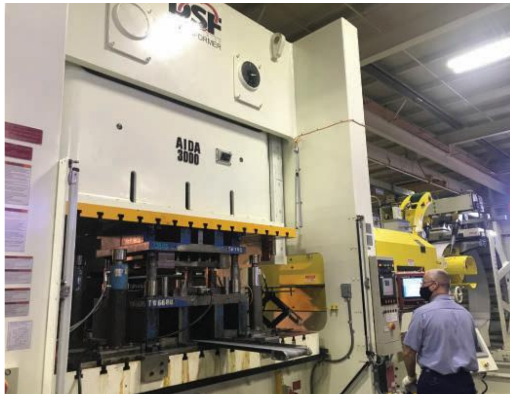
The stamper bought an AIDA DSF-N2-3000 330-ton, floor-standing servo press. The reverse tonnage dropped to 18 tons immediately. Tool life was extended as well.
