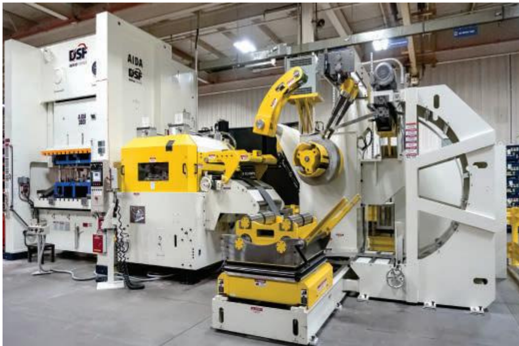
The stamper installed a Coe Press Equipment SpaceMaster Series 4 feed line, which fits into the limited footprint available.
