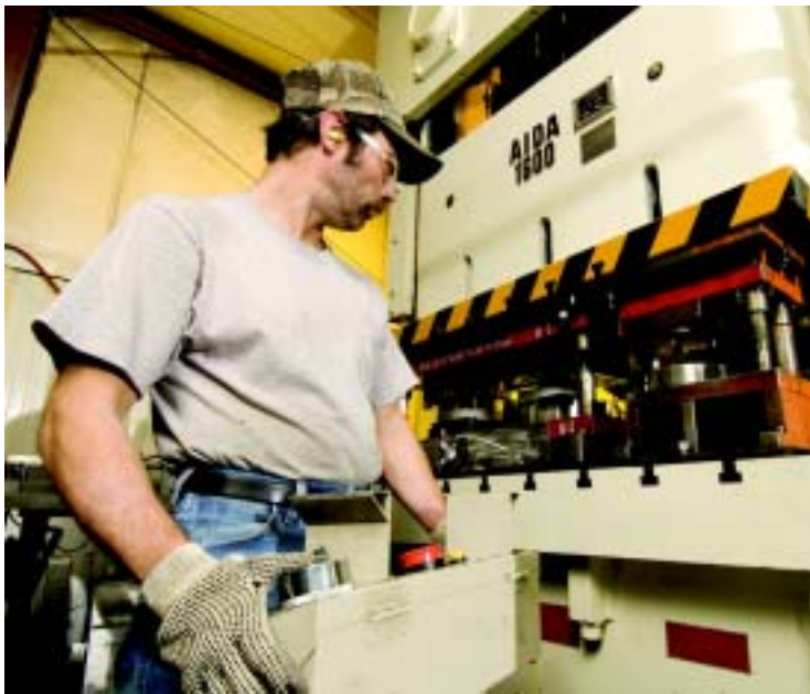
Being able to perform draw, progressive die and blanking operations all on one press is an advantage.
