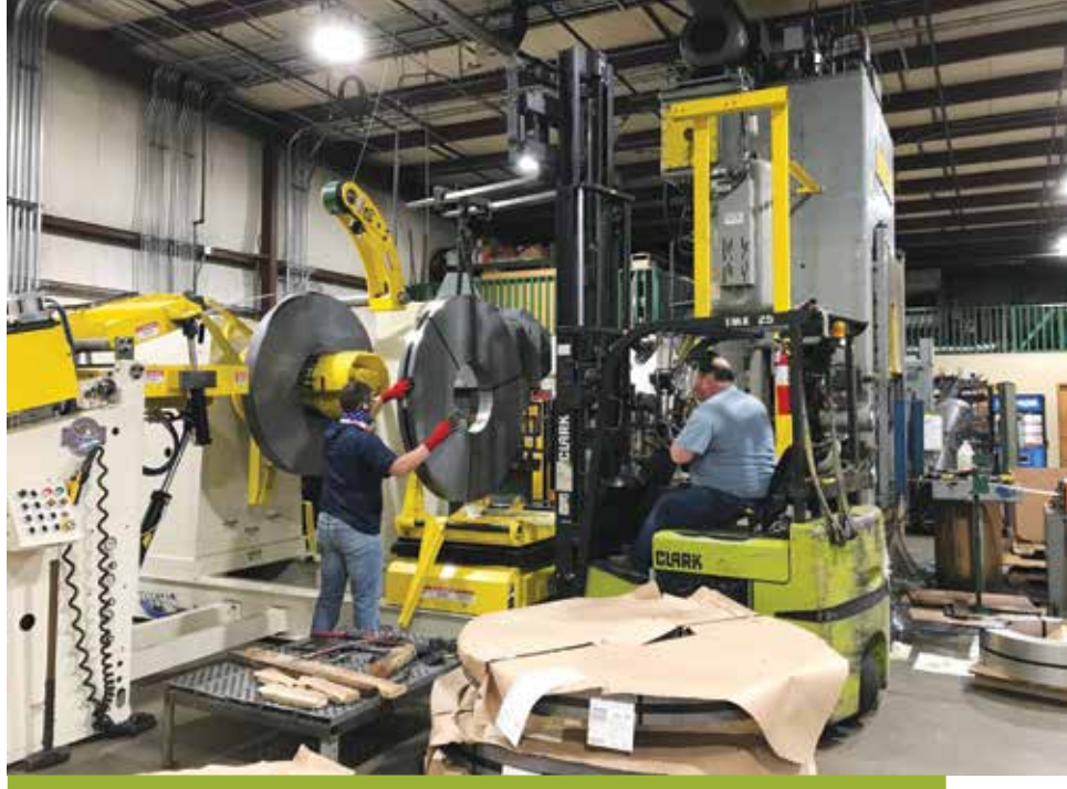
A 10,000-lb.-capacity feedline with coil car allows one coil to run while another is changed in minutes, above. Step-feed mode reduces die prove-out and setup time, left.
