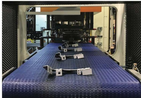
Installed and running in August 2019, the new press line at Engel Diversified features an Aida direct-drive servo press; a Coe Press 10,000-lb.-capacity servo-based coil-feed line; state-of-the-art press controls, with tonnage monitoring and signature analysis; custom part- and scrap-handling conveyor systems; and ANSI- and OSHA-compliant guarding.
