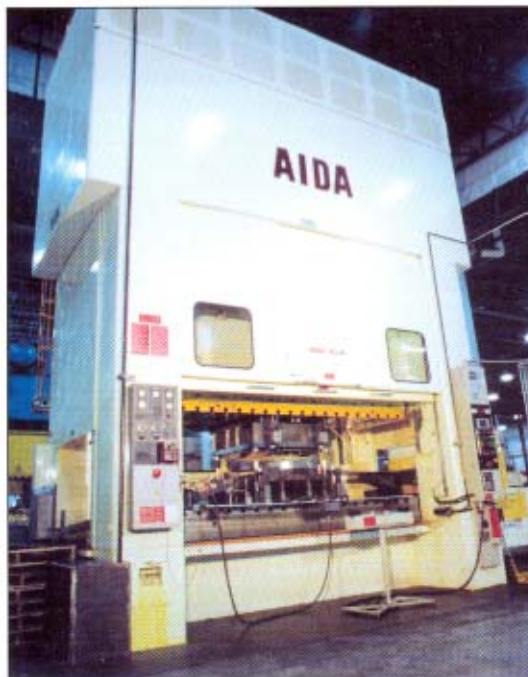
Kapco's automated press line is anchored by an Aida PMX 600-ton progressive-die press.
