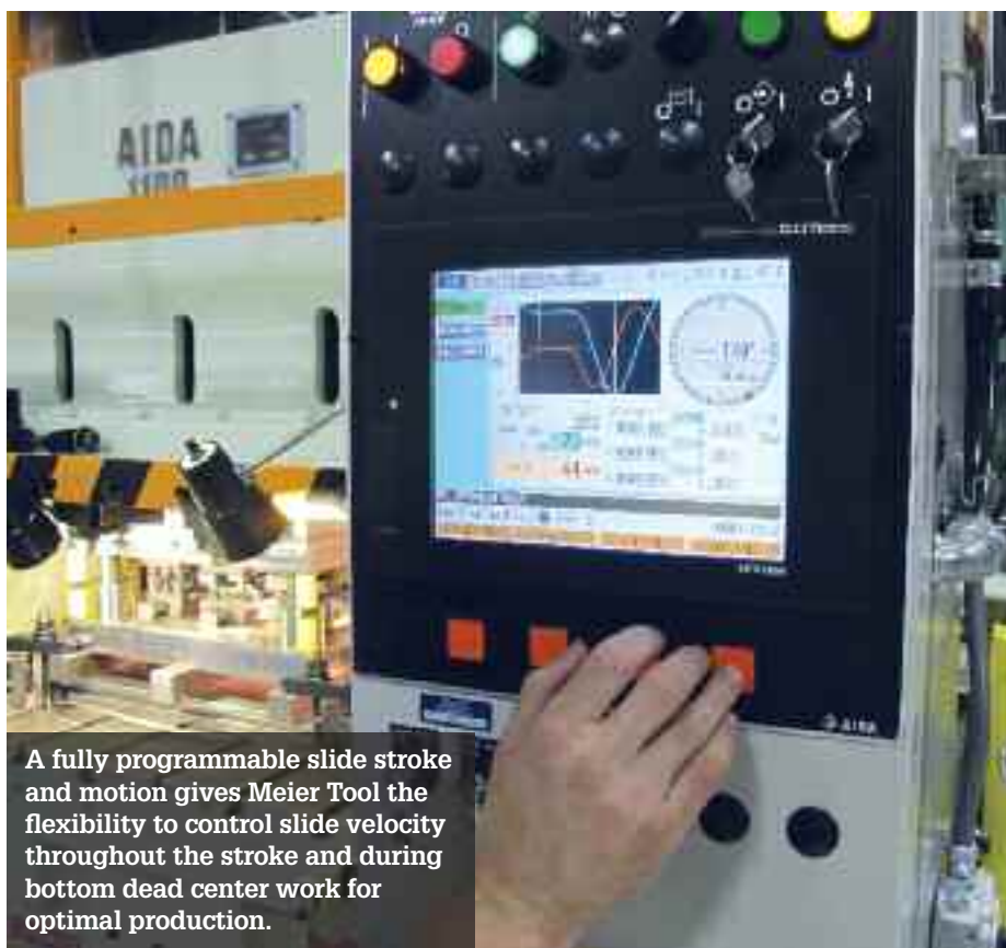
Meier toolmakers can see physically how a die is performing during different stages of the stamping process by using the servo press's manual step feed to test and debug complex tooling.
