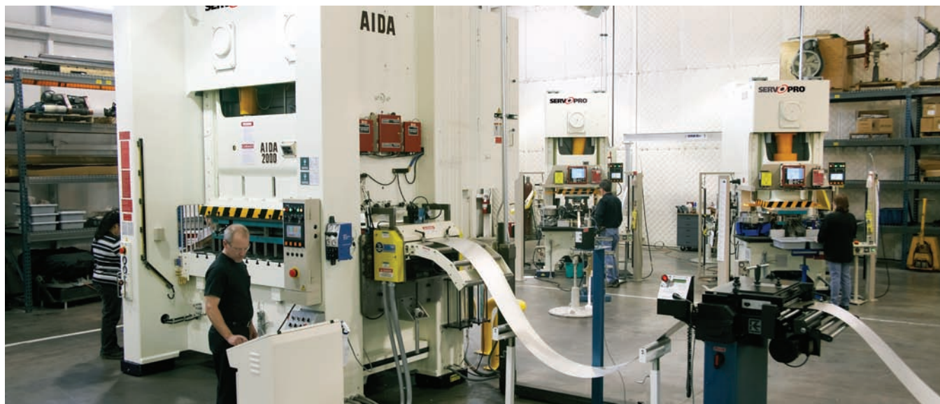
To take on progressive-die applications, Metalstamp added this ServoPro-equipped 200-ton straightside press. “With our conventional straightside presses, in-die assembly sometimes required our operators to stop a press to work on a tool,” says toolmaker and maintenance supervisor Terry Brown. “Each stop took minutes, but with the new presses, operators can perform the necessary tasks in seconds.”
