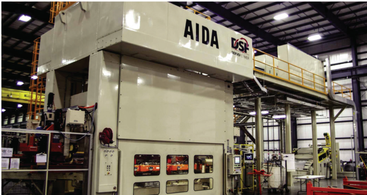
This 1500-metric-ton servo transfer press stamps a range of HSLA automotive parts. Among them, door-hinge parts, which were moved from production on a mechanical link-motion press to the servo press.
