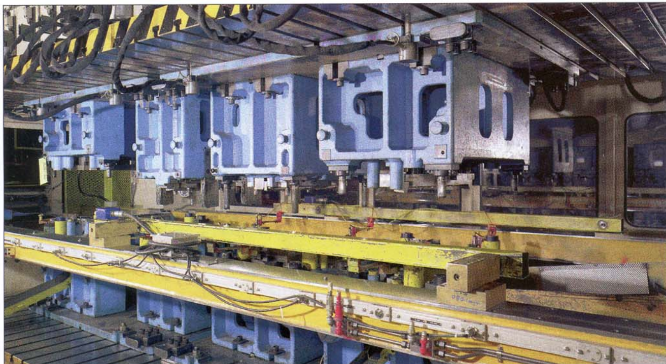
The TMX press at Midwest Stamping, Inc. boasts a bed capable of handling material to 72 in. wide, accommodating large progressive dies.
