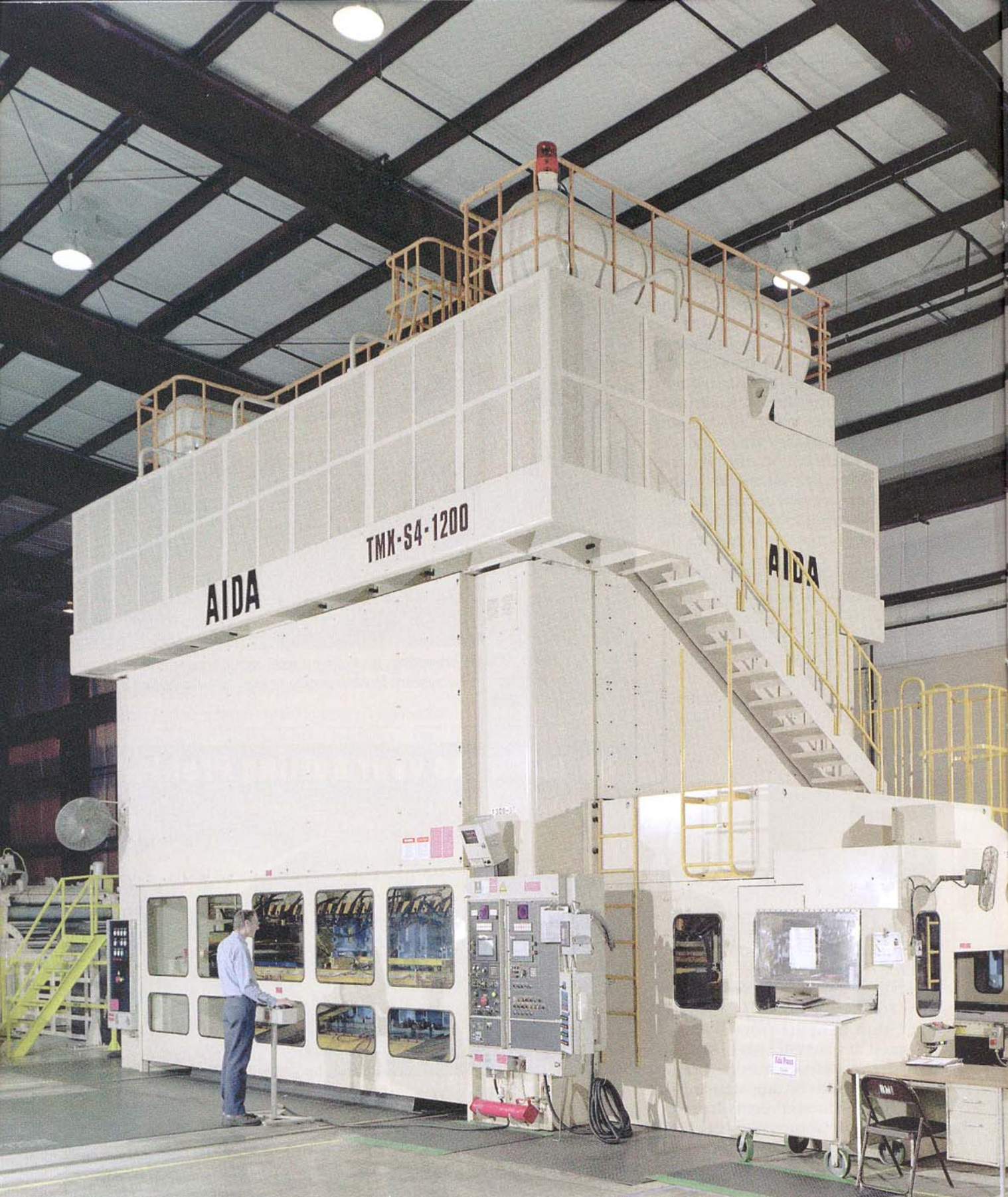
Midwest Stamping, Inc. installed this 1200-metric-ton Aida TMX electronic-servo transfer press in February 1999, in space built on to the firm's Edgerton, OH plant. Installed as a stand-alone work center, the press moved into high-volume production operating five days a week at 2.5 shifts and producing some 173,000 stampings per month.
