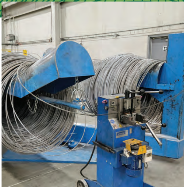
Omex designed a process for continuous wire feeding via welding automation. The wire makes its way through roll-forming and stamping machines to produce spindle parts for automotive applications.
