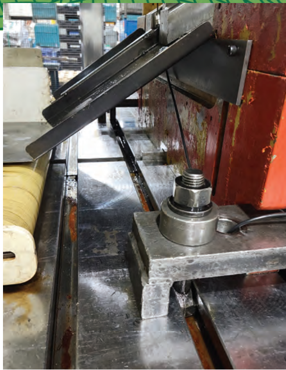
An Omex die-alignment innovation as shown on its newest 630-ton servomechanical press. Note how pressed grooves matched to die-block grooves and blocks (center of photo) are used to place tooling quickly and accurately.
