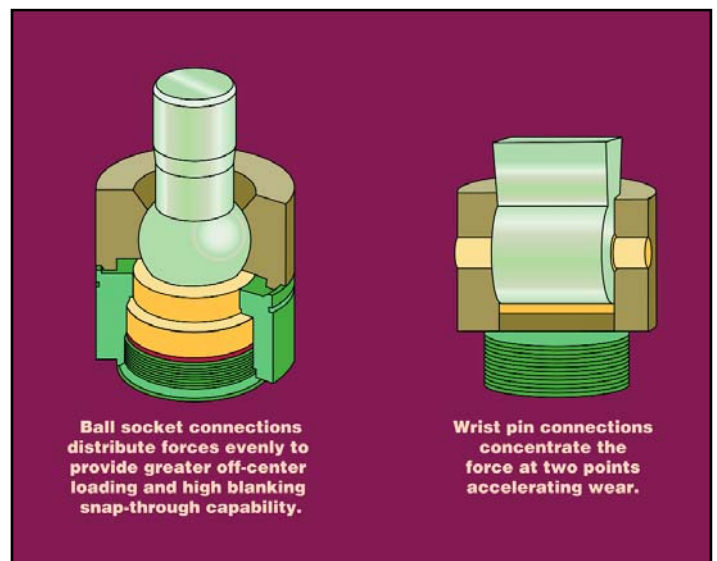
Fig. 2 Ball Socket Connection
