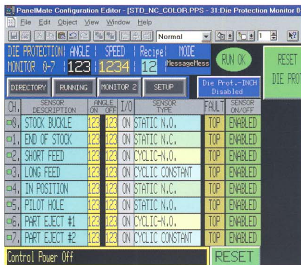
Figure 3. Access PLC-based control allows functions such as slide adjustment, slide counterbalance setting, and press speed to be performed automatically by job number.
