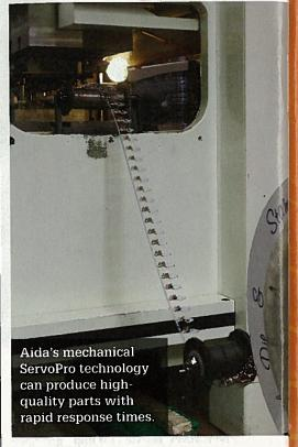
portant features for the manufacturer, the small footprint of the press and lower power consumption has proved to be an advantage. "Even with the large-capacity motors, the power supply requirement is significantly lower than that of a conventional press," says Mellinger. ServoPro capacitors store electrical energy when the servo motor is not under load. When the motor is loaded, power is drawn from the capacitors and not the main power supply.
