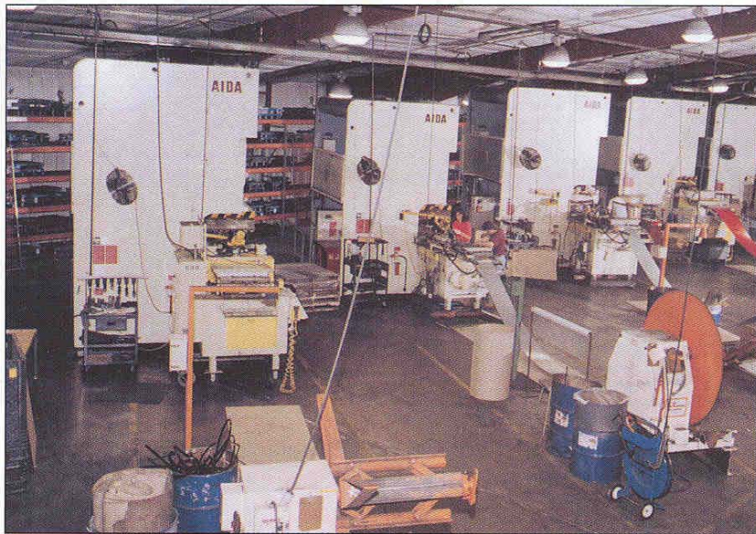
A portion of Tenere's line of automatically coil-fed Aida gap frame presses for use with progressive dies. Tenere Dresser has 17 presses ranging up to 275 tons capacity.
