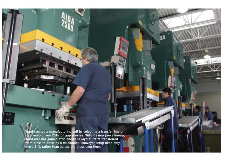
emergency markets and heavy-gauge, high-volume shaft-seal components requiring a tight-tolerance draw process. The press line stamps 0.090-in.-thick 1074 spheroidized annealed spring steel, stainless steel and draw-quality coldrolled steel. It runs one shift, five to six days per week depending upon customer requirements.
