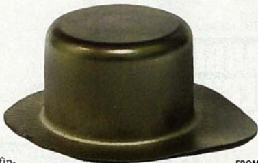
THE SIZE OF THIS DRAW FROM TITANIUM DEMONSTRATES THE FORMABILITY THAT CAN BE ACHIEVED WITH A SERVOPRO-DRIVEN PRESS.
