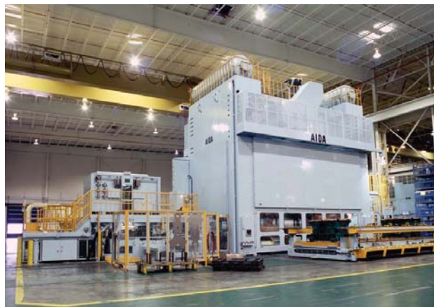
Transfer presses with eccentric load bearing capacity give stampers the flexibility they need in the design and layout of dies for production.
