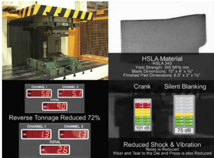
Fig. 6—Moving this blanking die to a servo-driven press allowed the use of a silent blanking-motion profile that reduced forward tonnage by eight percent, reverse load by 72 percent and noise level from more than 100 dB to just 75 dB. As a result, die life more than doubled and negative effects of reverse tonnage were nearly eliminated.
