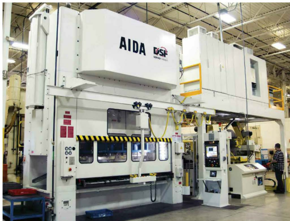
Servo-driven presses employ technologies such as capacitors and smart systems that efficiently manage energy use, helping to provide improved returns on investment.
