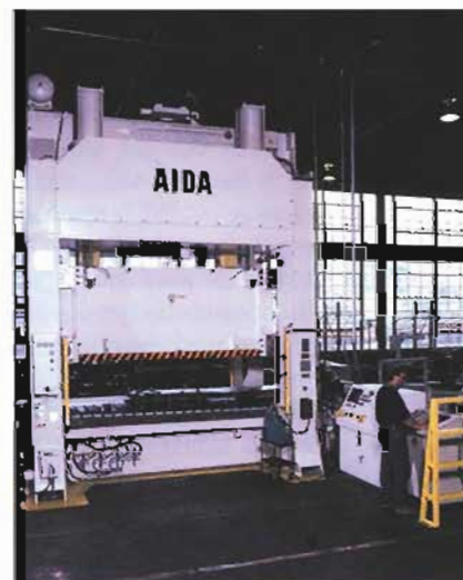
AIDA's tie-rod straight-side NST Series press was designed specifically for general purpose and utility work and offered Empire Comfort Systems high quality at a cost-effective pricepoint.
