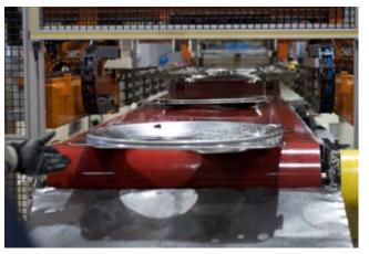
The Flextronics NST can accommodate up to seven dies on a bolster and transfer the part up to seven times. A variable position exit conveyor on the final transfer station is integrated with safety interlocks on the press control to allow the conveyor position to be linked to specific part numbers with specific numbers of stations.
