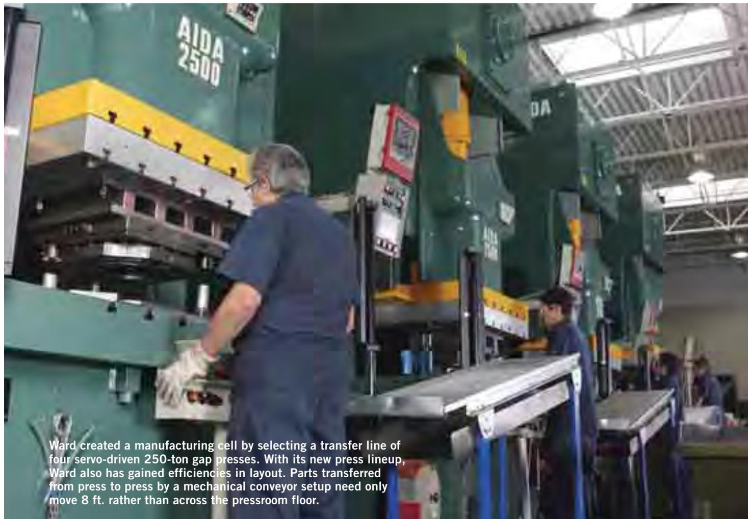
Ward created a manufacturing cell by selecting a transfer line of four servo-driven 250-ton gap presses. With its new press lineup, Ward also has gained efficiencies in layout. Parts transferred from press to press by a mechanical conveyor setup need only move 8 ft. rather than across the pressroom floor.
